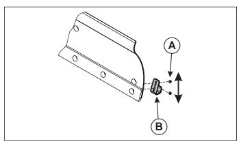
Figure 3. Skid Shoe Adjustment
